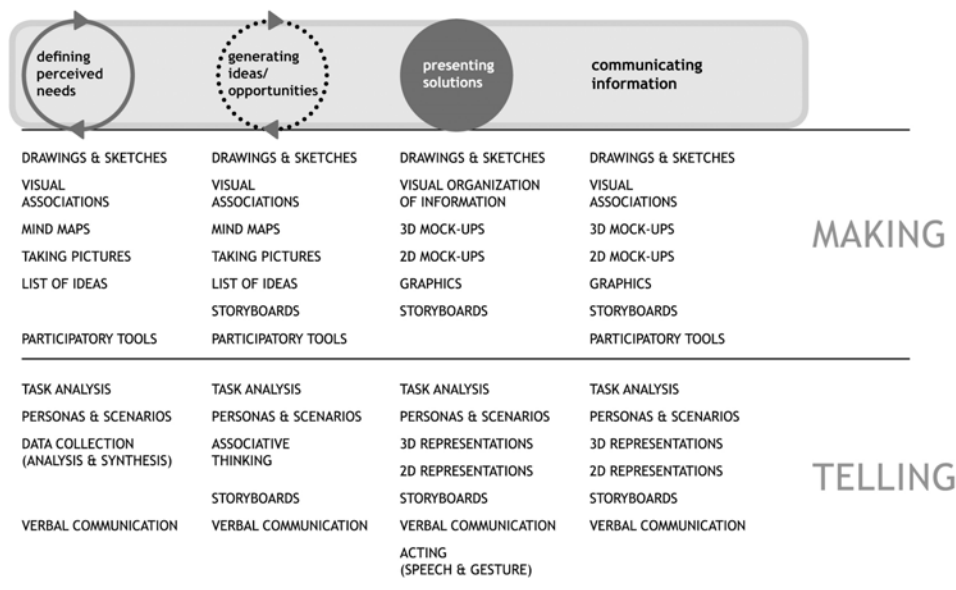
Figure 5 Visualization tools used at the beginning stages of the design process within multidisciplinary teams.
