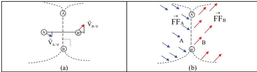
*Figure 3: The dualism between joint velocities in a mechanism and the face forces in the dual truss. (a) The primal mechanism and its linear velocities. (b) The corresponding dual truss and its face forces.*
