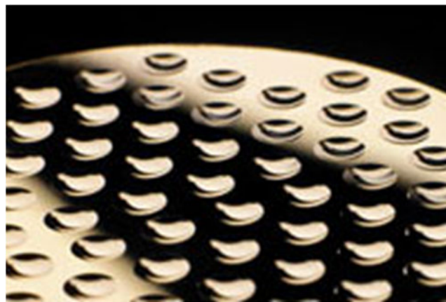
Figure 7. Detail of glass moulding mould for wafer based glass moulding [Webpage of Kaleido 2013]
