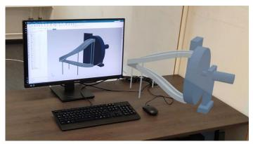
Figure 3 Augmented reality photo showing a mock-up of the hybrid AR computer workstation. An exported triangulation of the CAD model is shown on the HoloLens 2 using the built-in application *3D Viewer*.
