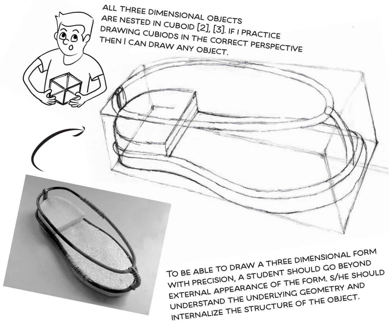
Figure 4. Visualizing an imaginary cuboid to sketch the object
